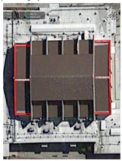
Please note that ALL of the parapet walls shall receive new metal CAP flashing.
